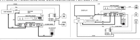
Sample setups to indicate the basic configuration for proper connections. Protecting all AC and signal lines will keep your system safe and ensure compliance with Panamax's Connected Equipment Policy.
