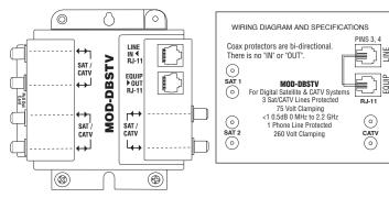
The MOD-DBSTV module provides protection for 3 SAT / CABLE / ANT and 1 telephone line.
