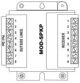
The MOD-SPKP module is designed to protect outdoor speaker, keypad, control and security wires (8 wires or 4 pairs). Equipment lines that lead outside the building are pathways for surges (sometimes called backdoor surges) to enter the equipment. This is why the lines FROM the outdoor equipment is connected to the LINE side of the module and the EQUIP side of the module is connected to the equipment.
