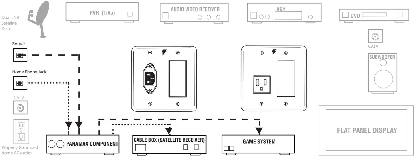
2. Connect component signal line cables (coaxial and 12V trigger). See tech brief for details.
