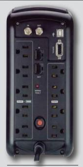
**RESETTABLE CIRCUIT BREAKER** Provides overload protection.
