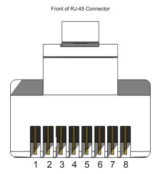
Gefen recommends the TIA/EIA-568-B wiring option. Use the following table when terminating cables in the field.
