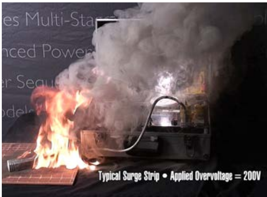
Standard power strips are not equipped to handle sustained over-voltage conditions.
