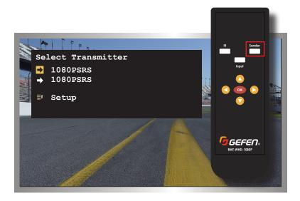
4. Press the ▼ and ▲ buttons to highlight the desired Sender unit.
