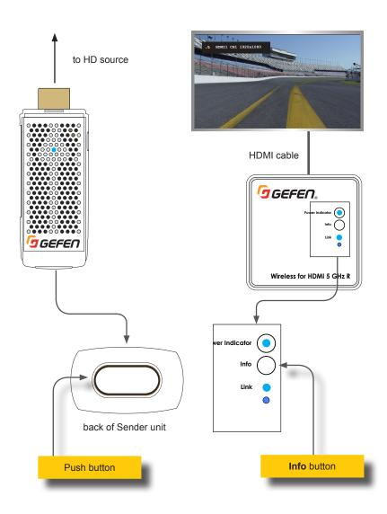
Information, similar to the following, will be shown on the display connected to the Receiver unit.
