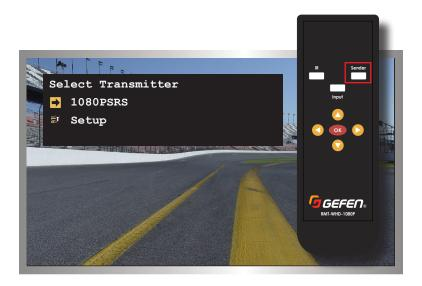
7. Press the ▼ button on the IR remote control to highlight the **Setup** option.
