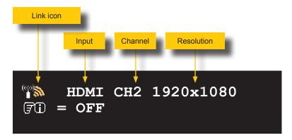
The **Link** icon indicates that the Receiver unit is connected to the Sender unit and is passing A/V data. See LED Indicator Messages (page 33) for more information on status icons.
