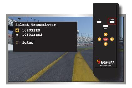
4. Press the ▼ button on the IR remote control to highlight the **Setup** option.
