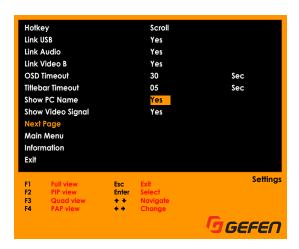
If the **Show PC Name** is set to **Yes**, then the name of the PC will be displayed above the current input resolution. This is the default setting.
