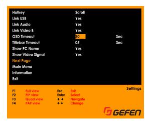
Select the desired timeout by using the ◀ or ▶ keys.
