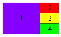
Displays all four sources on a single screen: The *main* (larger) window and 3 *subordinate* (smaller) windows. The *main* window can "swapped" with any of the *subordinate* windows.
