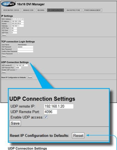
Sets UDP remote IP and remote port. Also enables or disables UDP access to the matrix. Click the Save button to apply changes.
