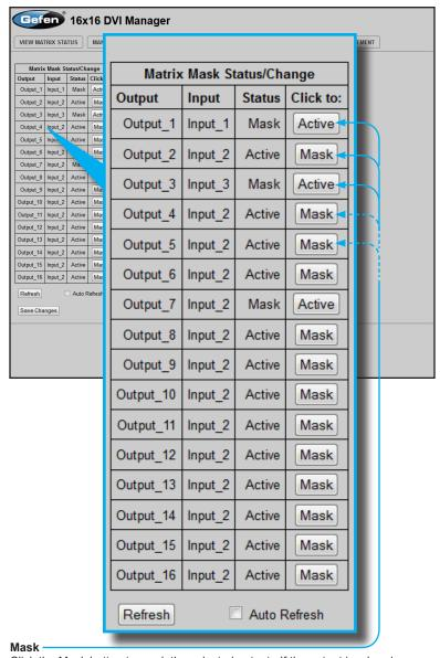
Click the Mask button to mask the selected output. If the output is already masked then the button will read "Active" (enabled). Click the ("Active") button again to toggle the masking state to "Mask" (disabled).
