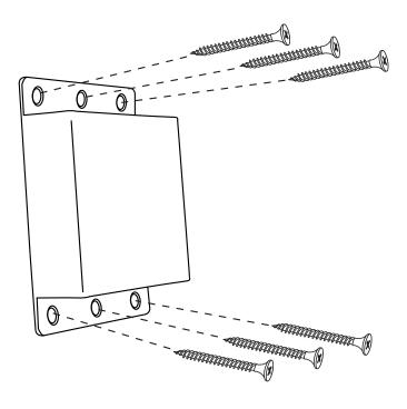
The Gefen *DisplayPort Extender over CAT-7* can be mounted on any horizontal or vertical flat surface (e.g. wall or inside / outside a cabinet with wood / drywall screws) as shown in the diagram above. There should be an inch or two of clearance between the edges of the unit and any walls or vertical surfaces to allow for enough clearance for connection and disconnection of the DisplayPort cable.
