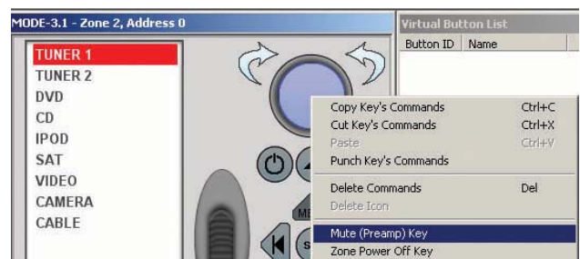
Figure 33 Placing The Zone/Whole/House Mute Command
