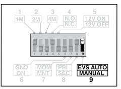
**DIP Switch position 9** is used to define how the CN-3600SE will recover from an Extreme Voltage (EVS) error. In some instances you may want the system to automatically recover once an EVS event has subsided, in other instances you may prefer to leave the system off until it can be manually restarted.
